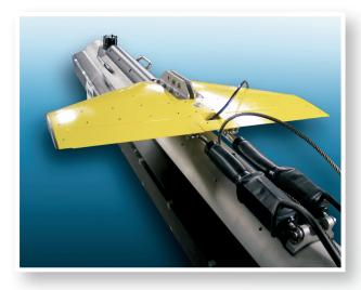
The K-Wing IV uses hydrodynamic forces to depress and steady the towfish while underwater. Dual ailerons are integrated and adjustable in software to compensate for roll bias and add fast-rise capability.
